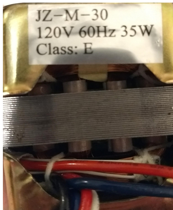
Figure 6-3: Fan Motor Connecting Wires
