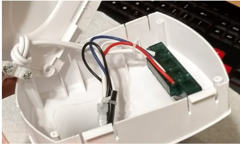
Figure 6-10: Oscillating Fan Switch Assembly
